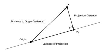
The above image serves as a useful visualization. Consider mean centered data. A data point has some fixed distance from the origin. We may consider finding a lower dimensional representation as either maximizing the variance of the projecting or minimizing the projection distance. The squared quantities must sum to a constant (the distance to the origin or original variance) thus minimizing one is equivalent to maximizing the other.
